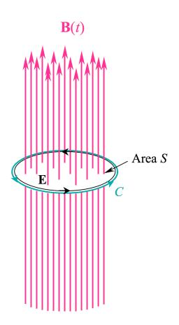
Current in the wire is caused by electric field,  $\mathbf{E}$ , that pushes the charge around the wire. In this illustration, the wire is removed, and the electric field remains. An integration contour, C, is also shown, that coincides with  $\mathbf{E}$ .
