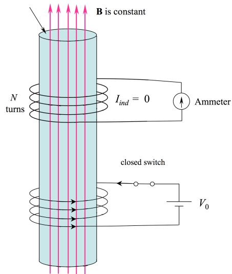
Once steady state is reached, in which **B** is at a constant value, the induced current is found to be *zero*.
