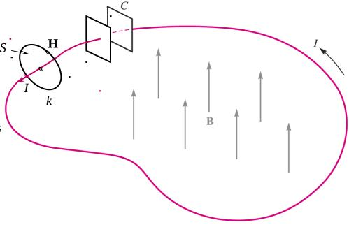
The integration surface is the flat plane whose perimeter is the circlular path, k. We assign the z direction (locally) to be along the current where it passes through the plane.
