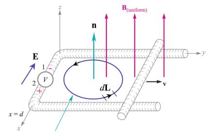
Direction of integration path of **E** through conductor (by right hand convention)
