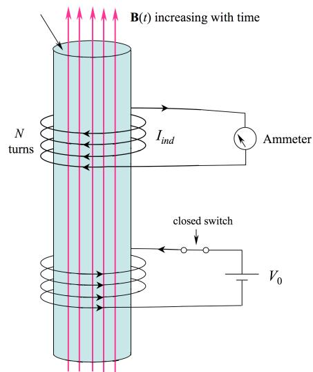
Closing the switch results in current that initially increases with time in the lower windings. Magnetic flux density  ${\bf B}$  is generated, which now links the upper windings; these are found to carry current,  $I_{ind}$ . This current exists *as long as*  ${\bf B}$  *increases with time*. Note the direction of the induced current and the position of the ammeter.
