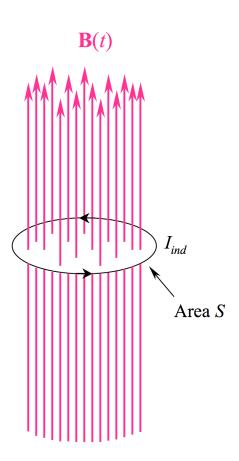
Consider a single turn of wire, through which an externally-applied magnetic flux is present. The flux varies with time.
