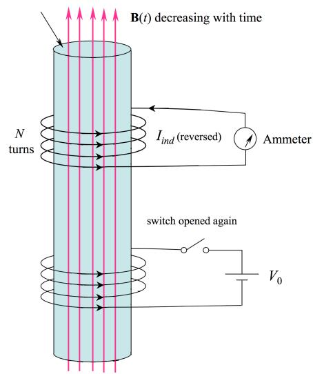
Opening the switch results in current that initially decreases with time in the lower windings. Magnetic flux density  $\mathbf{B}$  collapses, and the upper windings carry current,  $I_{ind}$  in the opposite direction from before. This current exists as long as the magnetic flux decreases with time.
